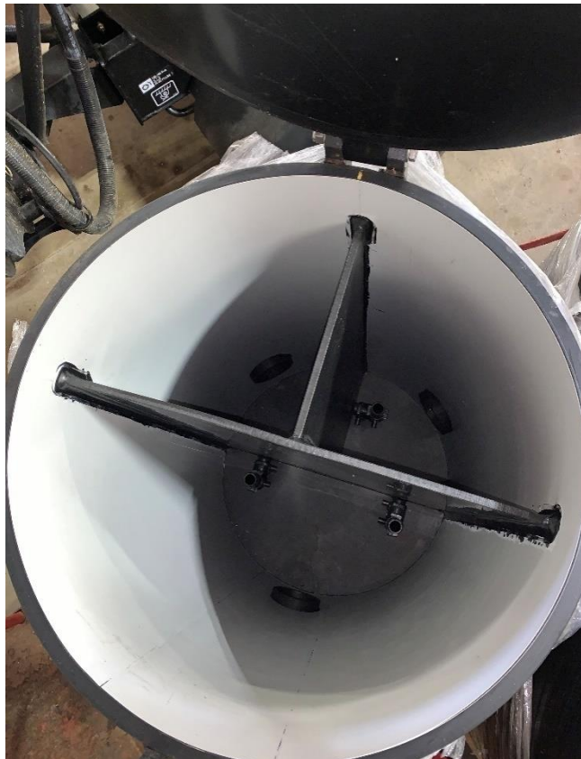
Figure 10. Interior of the Capillary hydroponic control basin prior to installation at the Capillary Hydroponic System and Variable Depth Rootzone research site at Michigan State University. The basin is divided equilaterally by a 0.91 m tall wall, then one half of the basin is divided again equilaterally by a 0.86 m tall wall resulting in a total of three chambers.
