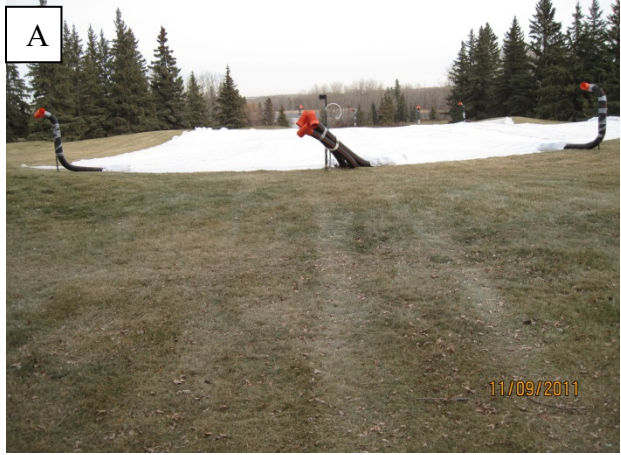
Figure 3- (A) Supplemental ventilation system (centre) and exhaust vents only (perimeter piping). (B) Diagram shows the configuration of the supplementary ventilation system with the 4 exhaust vents.
