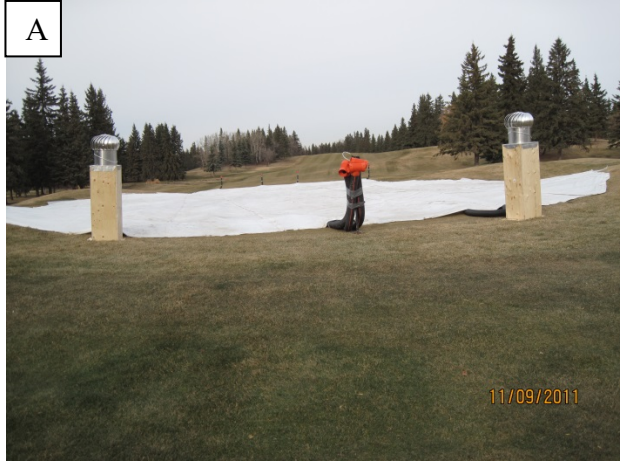
Figure 4- (A) Supplemental ventilation system (centre) plus “roof turbine” ventilation system. (B) Diagram shows the configuration of the supplementary ventilation system with the 2 roof turbine vents.
