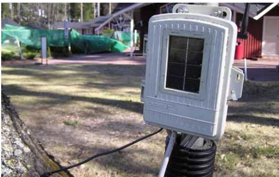
A thermometer to monitor the green soil temperature gives useful information. Photo Agnar Kvalbein, Messilän Golf
