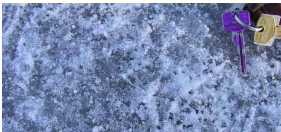
CMA penetrates the ice, but is not very efficient under low temperatures. Photo: Agnar Kvalbein, Bærum GC, February 2008.
