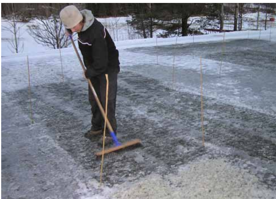
This ice was removed as a part of an experiment. The light green colour of the crushed ice indicates correct working depth. Photo: Agnar Kvalbein, Bærum GC, February 2008
